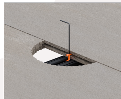
6 Use a 2.5mm Allen key to disengage and remove the clip.
