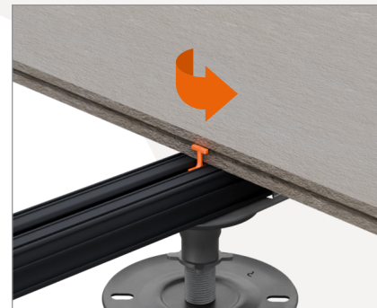
3 Slide T clip into the centre of the tile and rotate 90 degrees.
