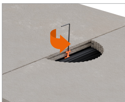
7 Rotate the clip 90 degrees until it aligns parallel with the tile joint.
