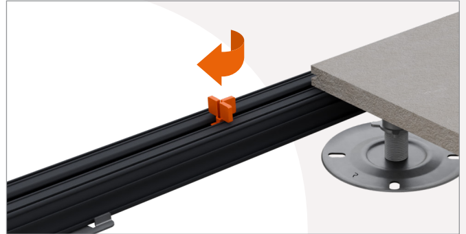
2 Insert the tile spacer into the upper groove of the joist and rotate 90 degrees.
