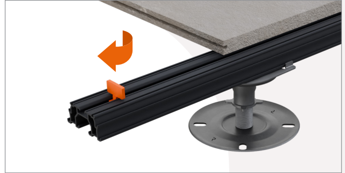
2 Insert the 2 way spacer into the upper groove of the joist and rotate 90 degrees.
